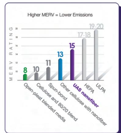
Figure 4 – MERV ratings compared with filter type
