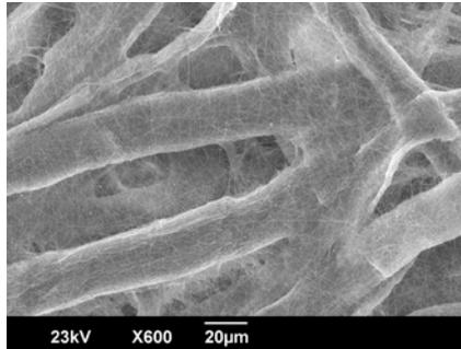
Figure 3 – UAS Nanofiber Filter 600x
